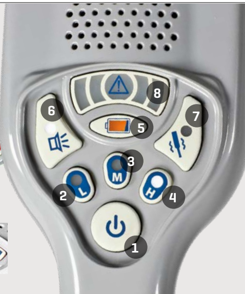
Optical indication proportional to the metal signal strength [Low, Medium, High].
