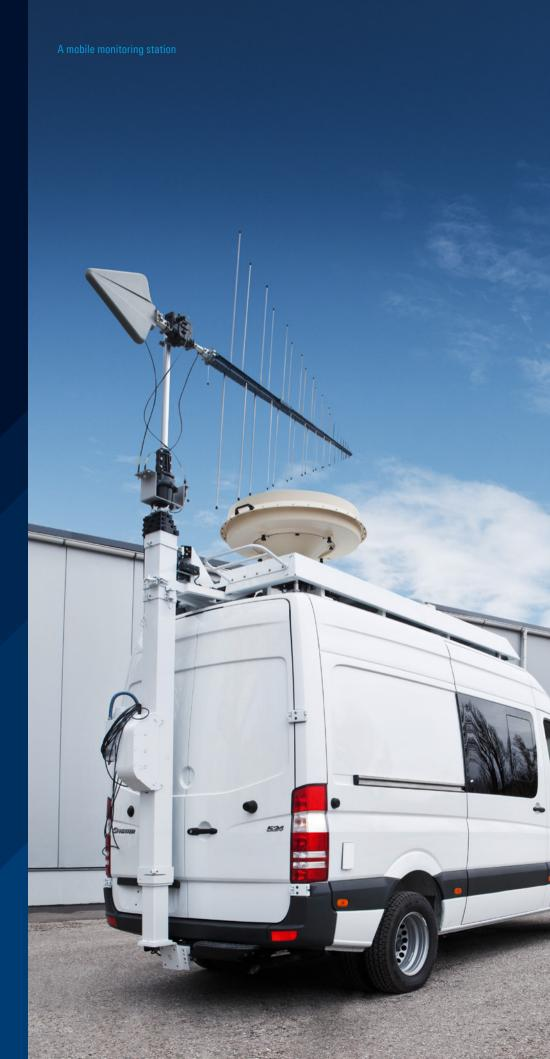
Operators of mobile stations work in a fatigue-free environment that features an ergonomic design. Facing frontward, operators can control the system while on the move, making it possible for them to provide instructions to the driver during homing and location tasks.
